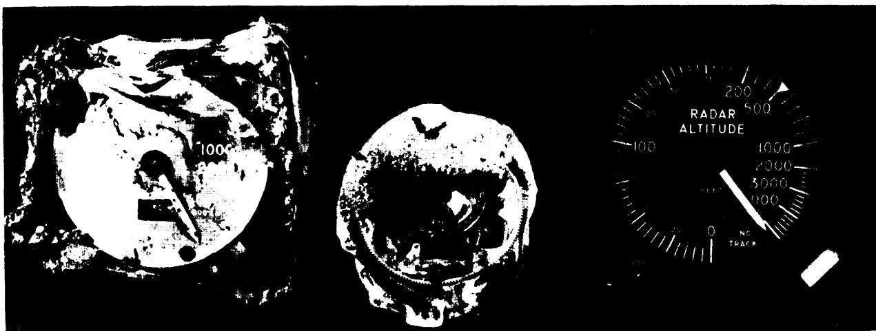
Figure 7-15. Instrument Analysis. Pilot's and copilot's radar altimeter, and new radar altimeter. Note both pilot and copilot indicators were set to 15, and both indicated no track conditions.
